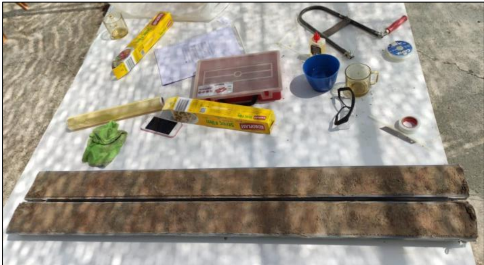
Figure 1.6. Split core samples
