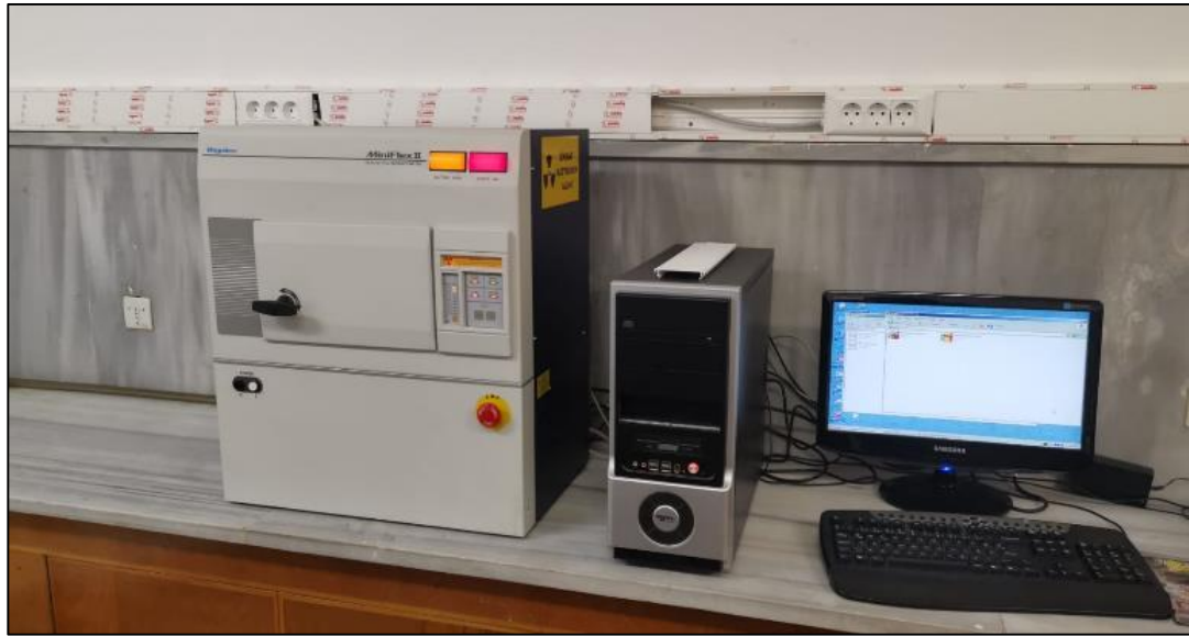
Figure 1.12. Rigaku Miniflex Benchtop Powder XRD device at the Department of Geological Engineering, Middle East Technical University
